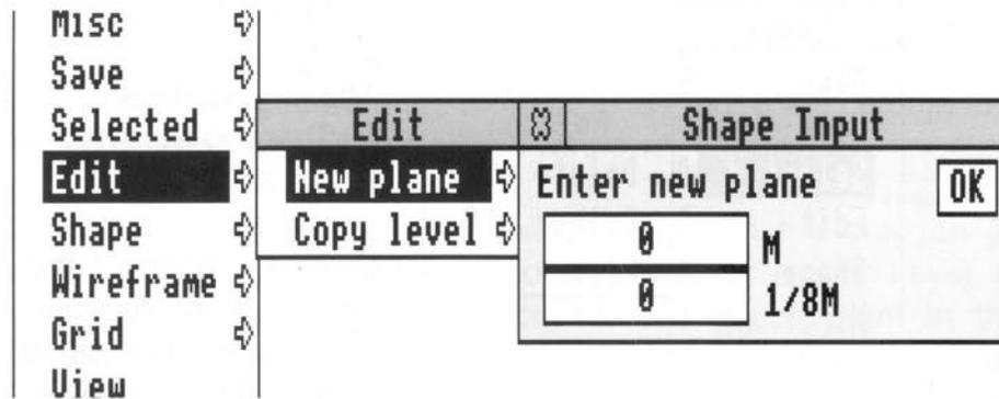
**New plane** creates a new working plane for point entry. Bring up the 'Enter new plane' window by following Edit=>New Plane=> and then enter the distance from the 0.000 plane that you want the new plane to be created at. The units are M and 1/8 M so to enter a new plane 1.5M from the 0.000 plane you enter 1 in the M box and 4 in the 1/8 M box.
